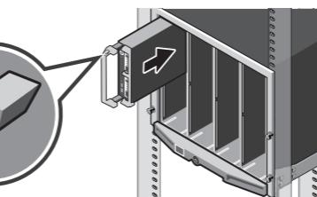
💡 NOTE: Beginning from the top, install the blade(s) into the enclosure, from left to right.
